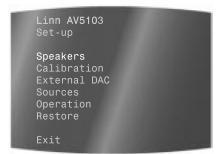
When you enter Set-up mode the sound from your system is automatically muted, except where test signals are played through the loudspeakers during some of the calibration options. In addition, any active record paths will be cleared.
