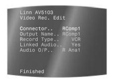
NOTE: You cannot change the connector used for an existing record output. If necessary, remove the record output and then define the record output on the connector you want to use.
