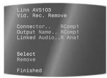
Select Remove to remove the record output, or Finished to exit from the menu without removing an output.
