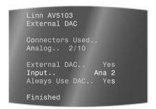
Select the Input menu option and set it to the analogue connector the external DAC is connected to.
