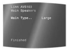
Set the Main Type to Large if the main loudspeakers are large with a full-range frequency response, or Small if the main loudspeakers are small and you want the main left and right bass to be handled by a subwoofer.
