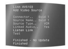
Set the Connector menu option to the analogue or digital audio connector used for the audio/video link.
