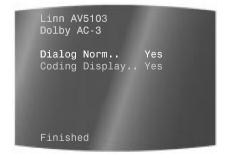
Set the Dialogue Norm option to Yes to compress sound levels around the normal dialogue range, or No to leave the relative signal levels unaltered from the original recording.
