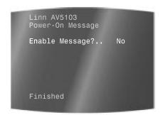
If set to **Yes**, the following information will be displayed on the System Controller's front panel when it is next switched on:
