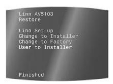
Select User to Installer to save the currently-defined set-up as the Installer set-up. A screen is displayed which prompts you to confirm your settings before proceeding to the next stage.
