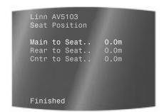
Enter the distance from the seating position to the main loudspeakers, rear loudspeakers, and centre speaker, using the Main to Seat, Rear to Seat, and Cntr to Seat menu options respectively.
