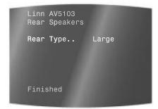
Set Rear Type to Large if the rear loudspeakers have a full-range frequency response, or Small if the rear loudspeakers have limited bass handling and you want the bass for the rear to be redirected automatically to another speaker.
