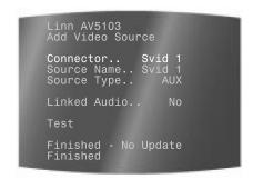
Press VOLUME - or + to step through all the unused connectors in the sequence SVID 1, SVID 2 (Svid inputs), Comp 1 to Comp 8 (composite inputs) and VSW 1 to VSW 6 (video switcher).
