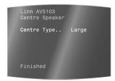
Set the Centre Type to Large if the centre speaker has a full-range frequency response, or Small if the centre speaker has limited bass handling and you want the bass for the centre to be redirected automatically to another speaker.
